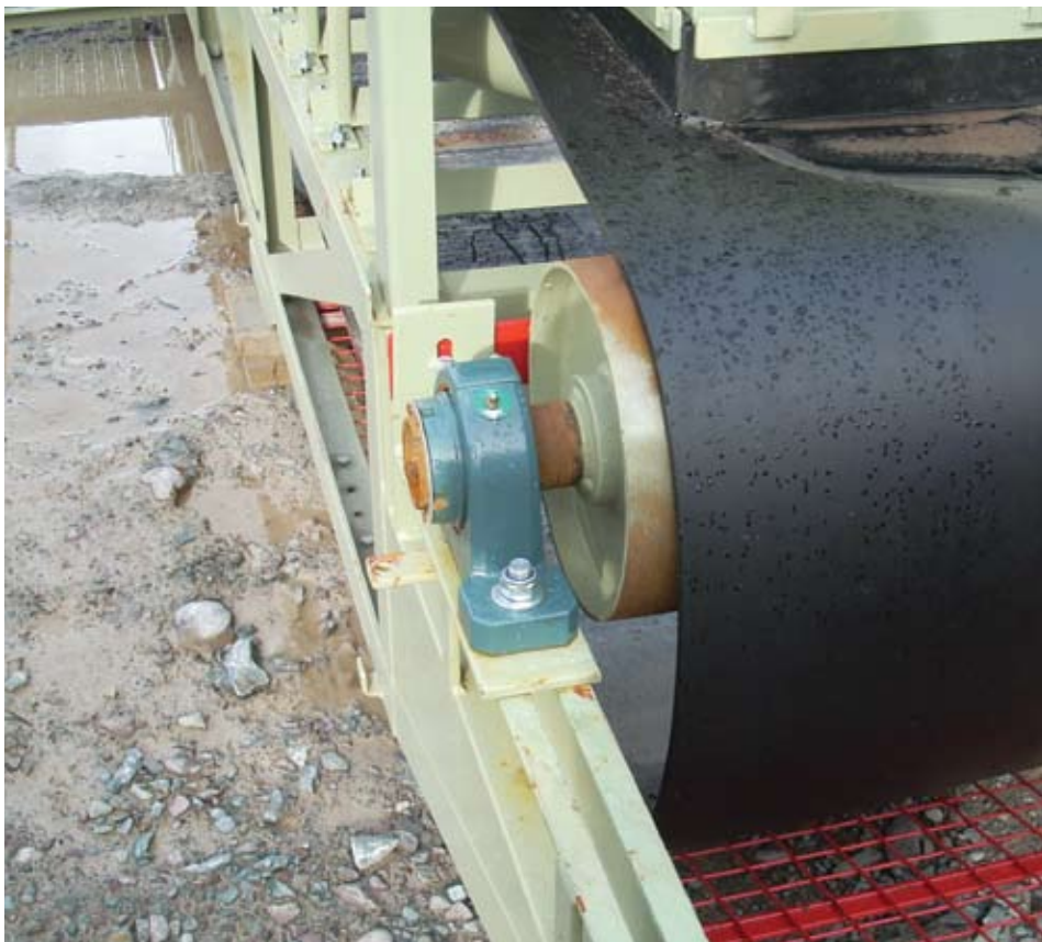
Dodge ISN bearings have helped increase reliability by around threefold at Corcoran Concrete's quarry.
