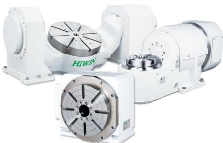
HIWIN Torque Motor Rotary Tables (TMRT) use a direct-drive torque motor, built-in high-rigidity and high-precision bearings, absolute encoders and powerful brake system to ensure excellent acceleration capabilities and high precision uniform movements. HIWIN TMRTs are backlash-free, optimized for high torques, have robust dynamics and are highly adaptive to the most demanding of automation processes.
